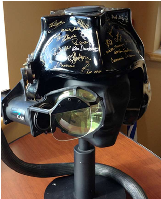
CAE's fiber-optic helmet mounted display created in the 80's. The ancestor of today's virtual reality lenses
