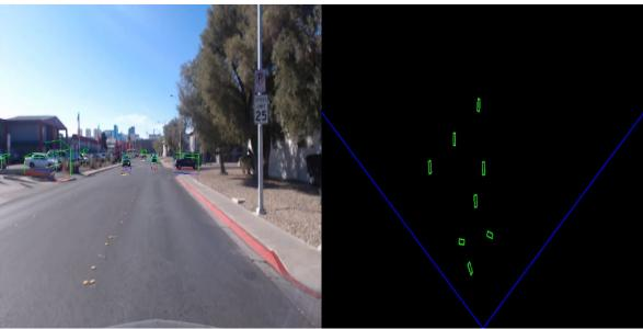
Figure 2: Monocular 3D detection. Left: dash cam image. Right: top-down bird's eye view of the scene.
