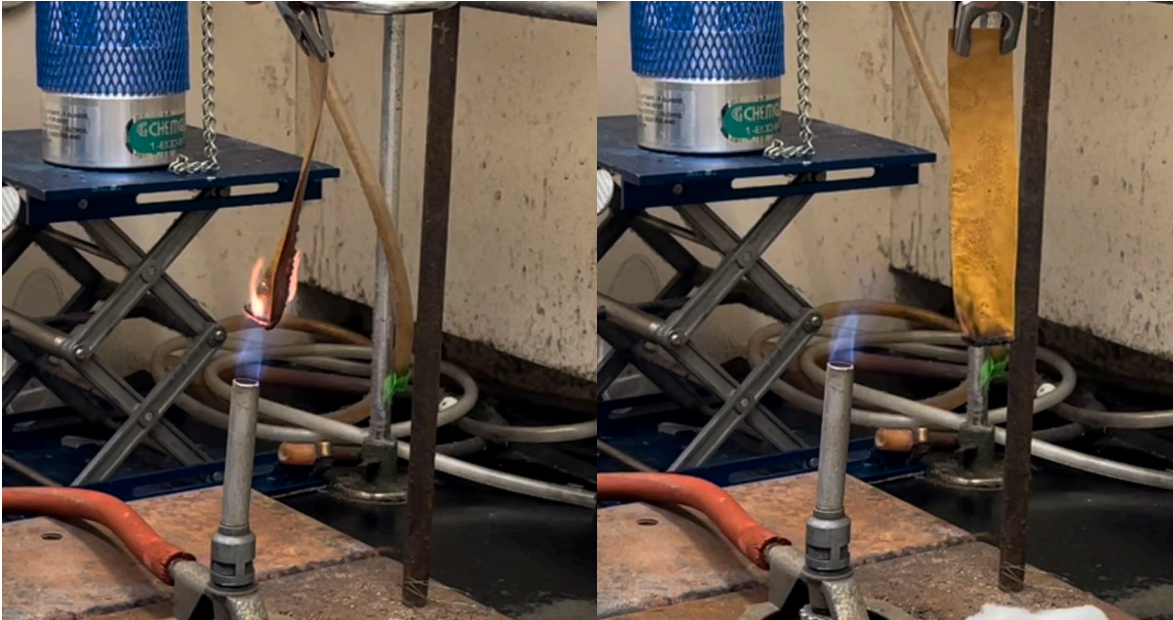
Figure 2: Test and Result After Two Burn Tests with 90° Bunsen Burner
